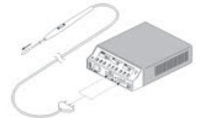
An adapter may be necessary to connect the pencil to generators not manufactured by Covidien. Refer to the *Surgical Products Catalog* for the appropriate adapter.
