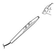
Ensure the insulating sleeve fits securely inside the nose of the pencil so that the nose overlaps the insulating sleeve by at least 1/8" (0.3 cm). 4. Hex electrodes have a depth indicator. The line on the depth indicator should be flush with the tip of the handswitching pencil.
