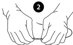
The needle is broken off at the score mark (Fig. 2) to create a connector pin (stainless steel electrode).
